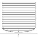
When retracted there should be 5-10mm clearance between front of basket and edge of base/top and inside of door face.
