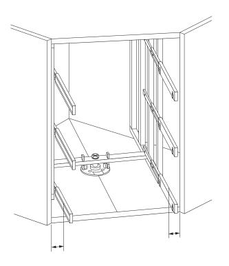
Mark and drill for top and bottom mounting discs. Fit screws.
