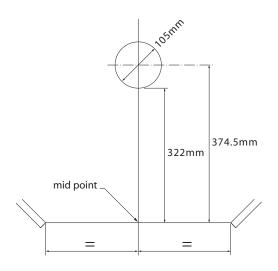
Insert carousel frame into base unit and align bottom mounting disc with pencil circle. Extend runners and adjust carousel position to ensure equal measurements between runners and cabinet sides.
