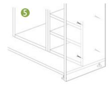
Scribe end panel into the back wall and ceiling. Fit top extender. Drill through and screw from internal carcass to fix securely.
