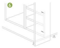
For wall-to-wall installations an end panel is not required. Fit the extender panels flush to the front of the base and fix by drilling through and screwing.
