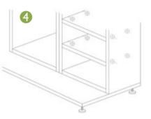
Assemble internal shelves, shelf stacks, drawer units and hanging rails using pre-drilled hole and cam and dowel assemblies.
