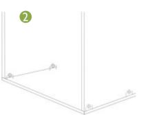
Assemble all internal carcasses using pre-drilled cam and dowel assemblies.
