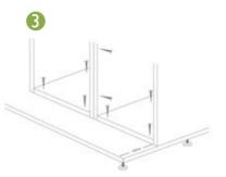
Align carcasses to the rear of the base. Drill and screw carcasses to the base and to each other.
