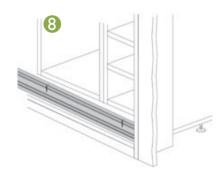
Fit top track flush to top extender by drilling and screwing. Bottom track is set back 9mm\* from the front edge of the base.
