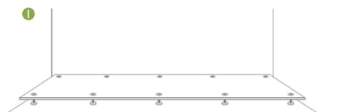
Screw legs into base, place base into required space and level accordingly. NB:Additional packing may be required under legs for very uneven floors.
