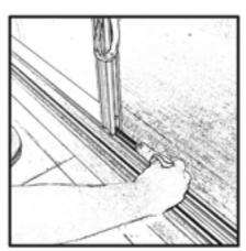
The door height can be adjusted using a screwdriver
