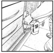
Screw bottom track into place 12mm back from front edge of wardrobe frame.
