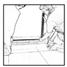
Fitting the rear door first, lift the door into the top track at a slight angle before guiding the bottom wheels into the bottom track.
