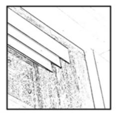
1. Screw top track into place flush with front of wardrobe frame.
