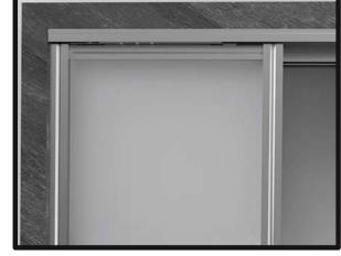
2. Close the door fully. This will push the soft close plate into the correct position within the track. If the plate does not meet the soft close on the door, adjust the door height using the adjustment screws at the bottom of the door.
