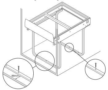
2 Before permanent attachment to the cabinet base, fit containers and lid and test for ease of opening and container removal. Ensure the unit is clear of door hinges and other obstructions during operation.
