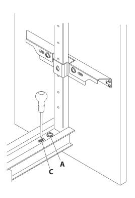
**11** Adjust the horizontal and lateral door alignment with screws on the door brackets.
