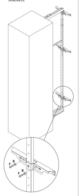
8 Offer door to frame. Mark and fix screws in two positions.
