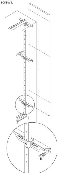
**9** Adjust vertical door alignment with the 3 door bracket screws.
