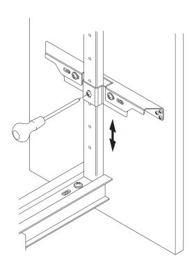
10 'Fine' adjustment of the vertical alignment of the door can be achieved by loosening screw A and adjusting screw C.
