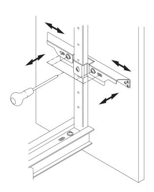
12 Attach the frame basket clips to the frame and position the baskets. Attach basket locking clips to secure baskets - snap fit connection.
